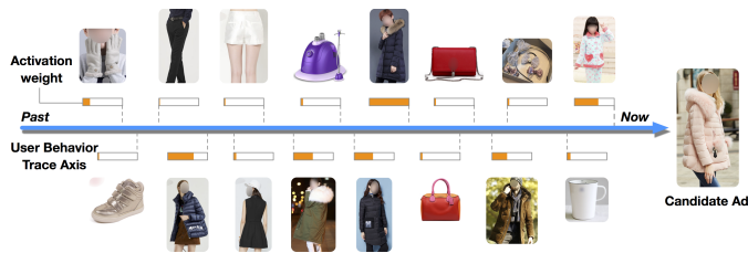
Figure 5: Illustration of adaptive activation in DIN. Behaviors with high relevance to candidate ad get high activation weight.
